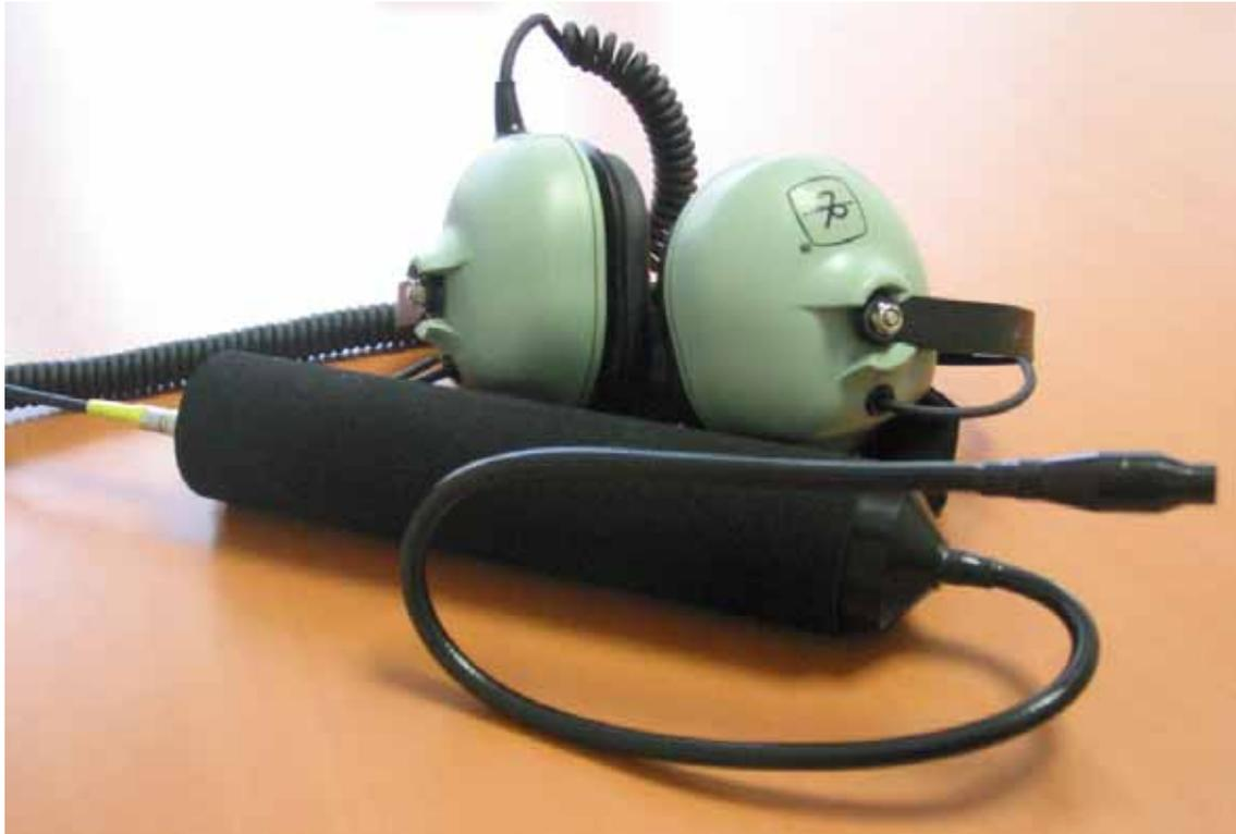
**The PSX-GN is a state of the art ultrasonic leak detector with dual converters.** It has a sealed body not affected by dust, sand, oil, water or other contaminants (\*).
