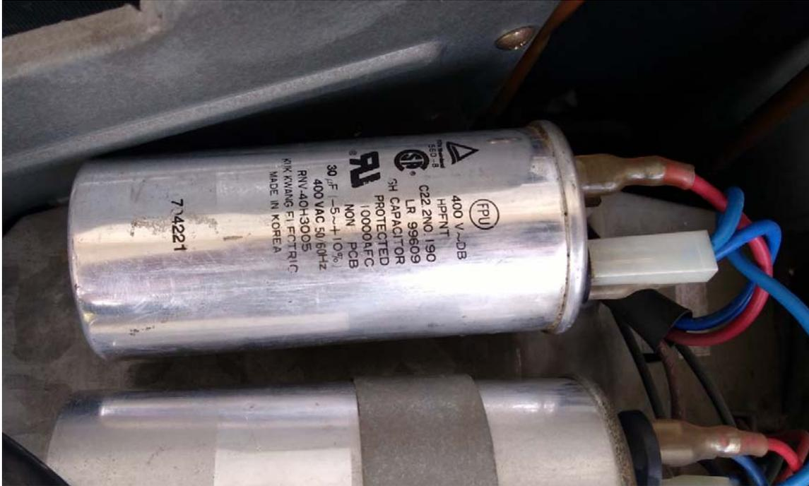
The capacitor we measured was listed as a  $30 \mu F$  -5% to +10%.  $22.89 \mu F$  is 23.7% below the  $30 \mu F$  listed on the capacitor whose lowest value (the -5% of 30) is  $28.5 \mu F$ .
